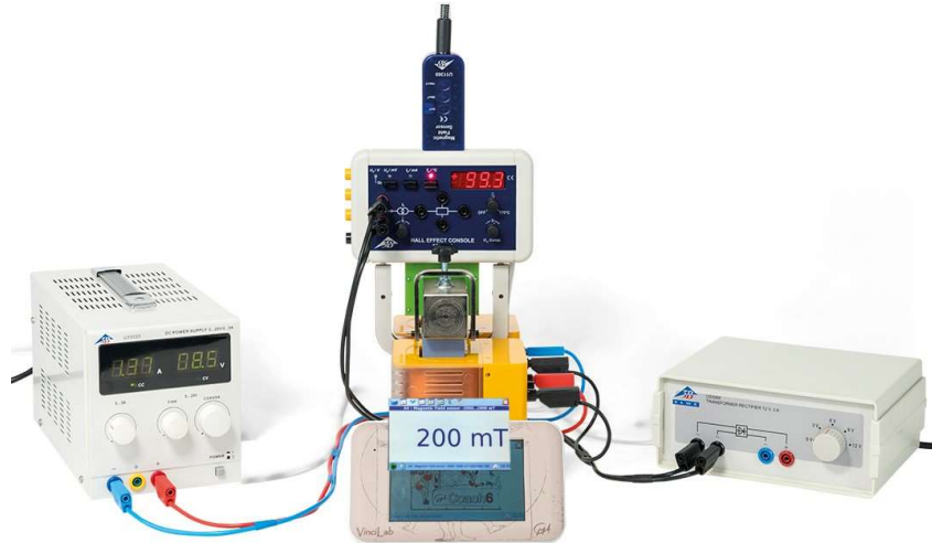
Fig. 9: Experiment set-up for investigating the Hall effect with a uniform magnetic field
