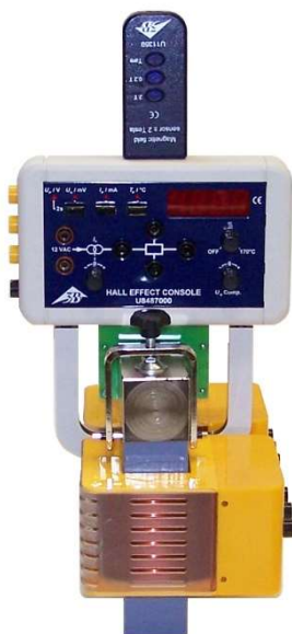
Fig. 8: Set-up with magnetic field sensor, front view
