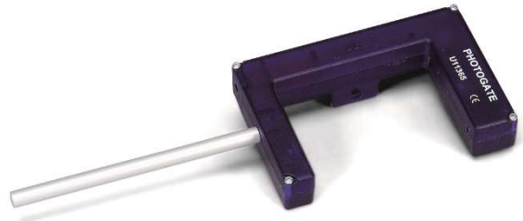
Fig. 1: With stand rod and any kind of stand apparatus, e.g. for experiments with air track
